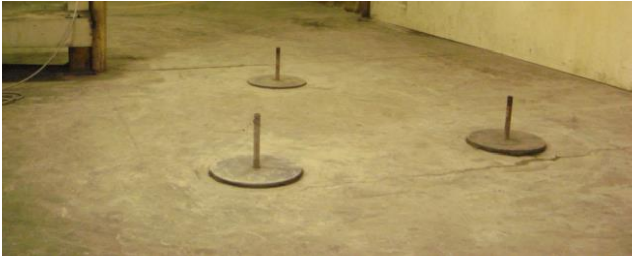
PHOTO#7 Piles showing the caps after testing.
